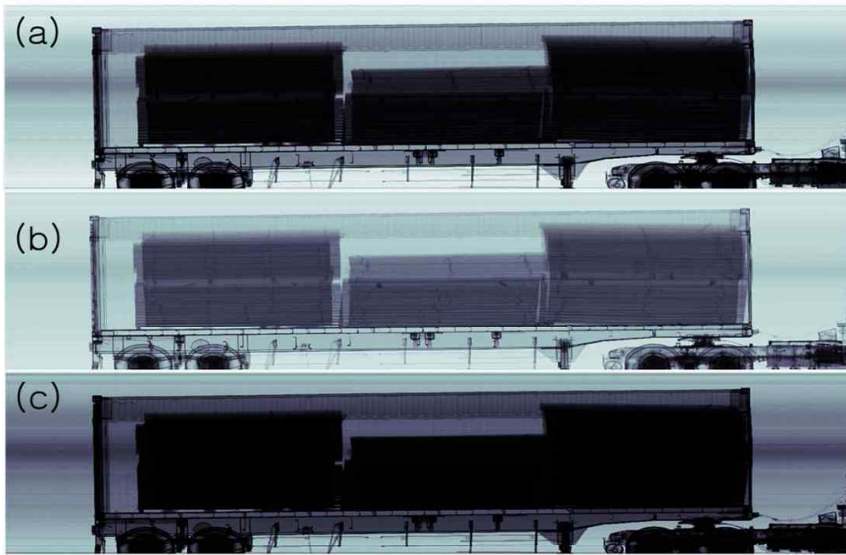
Figure 29. Results of post-processing image by gamma factor : (a) Original image (b) Controlled image with gamma factor greater than 1 by slice bar (c) Controlled image with gamma factor less than 1 by slice bar
