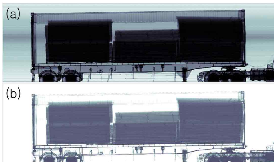
Figure 28. Results of post-processing image by window width/level : (a) Original image, (b) Post-processing image
