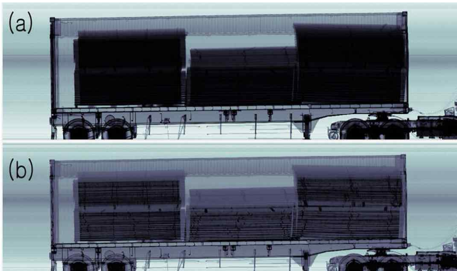
Figure 30. Results of post-processing image by histogram equalization : (a) Original image (b) Controlled image
